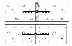
**Earth Shield JP211** Rear Guard - waterstops are ideal for flat pavement jobs such as runways and large containment slab's etc.
