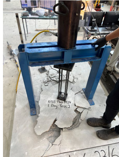
b) Concrete cone failure
