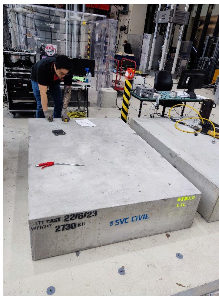
a) Slab before installation of anchor
