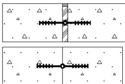
**Earth Shield JP211** Rear Guard - waterstops are ideal for flat pavement jobs such as runways and large containment slab's etc.
