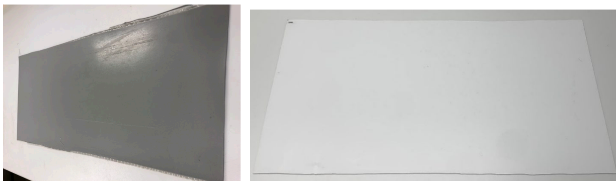
FIGURE 2 UNDERSIDE OF NITOPROOF 910 - WATERPROOFING MEMBRANE
